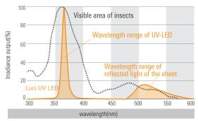
Highly initial UVA output at 365 nm is most attractive spectrum for flying insects. Almost invisible with eyes of human being.
